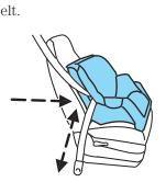
be no more than one inch (2.5 cm) of movement for proper installation.
